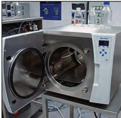
your autoclave is not working properly and needs immediate service. Autoclaves should be spore-tested every 100 to 200 hours of full-pressure use. For most clinics this is about twice a year. The cost for the spore strip culture will be \$24. If the strip gets wet or damaged prior to autoclaving it could yield a false positive result and should not be used.
